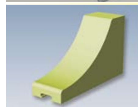
Edge curler Operation on the fourdrinier machine in paper industry
