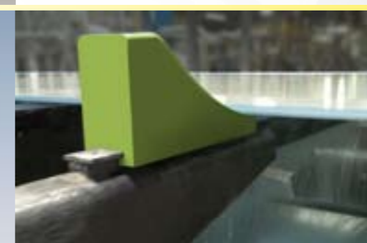
Edge curler Operation on the fourdrinier machine in paper industry
